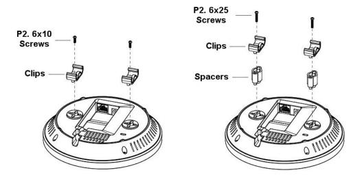
2. Press the device into the ceiling T-rail until the clips snap securely into place.
