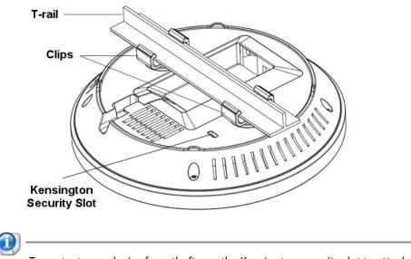
To protect your device from theft, use the Kensington security slot to attach a cable lock (not included).
