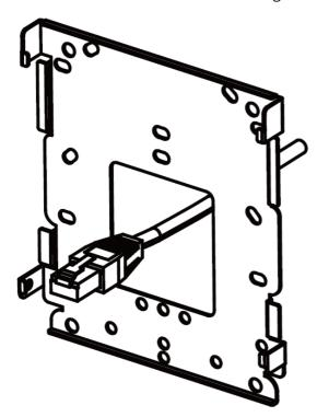
3. Align the mounting bracket with the outlet box and attach the mounting bracket with the original cover screws. We recommend you use flat-head screws to make sure the access point is flush with the wall after installation.
