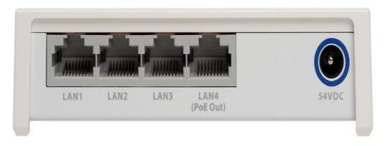
You can enable and configure these ports in the device configuration in WatchGuard Cloud. For more information, go to Configure Access Point Network Interface Settings.
