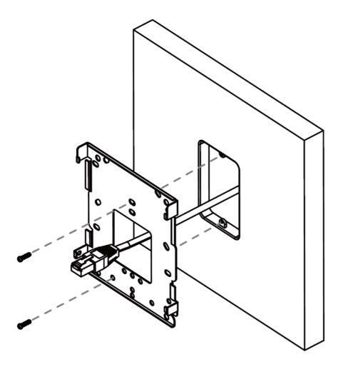
4. Connect the Ethernet cable from your network to the PoE+ IN LAN/Uplink port on the rear panel of the access point before you attach the device to the mounting bracket.
