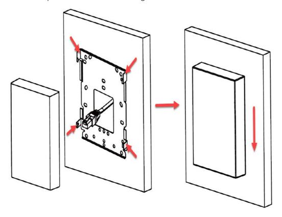
5. Insert the included bracket screw on the side of the access point to secure the device to the mounting
