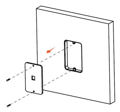
2. Pull the Ethernet network cable through the center of the mounting bracket.
